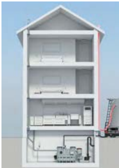
Separate pendulum gas pipe above the roof
