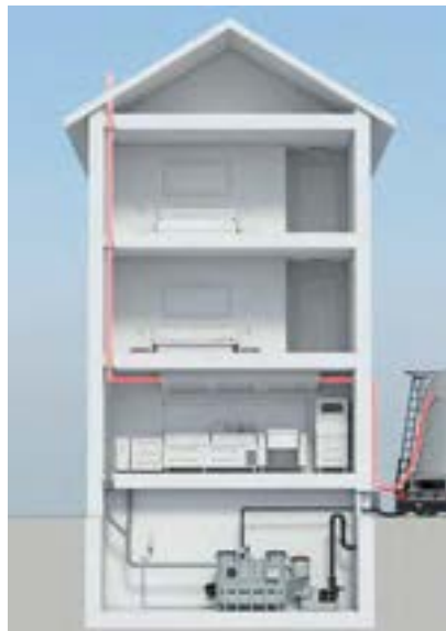
Pendulum gas line connected to ventilation line of grease separator
