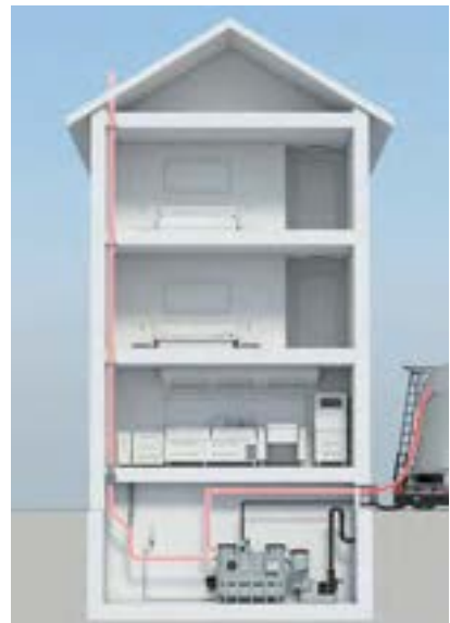
Pendulum gas line connected to grease separator
